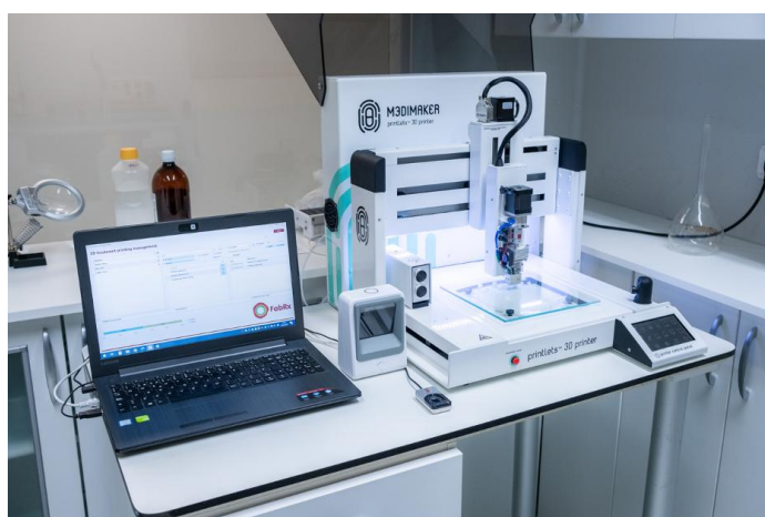
Fig. 3. FabRx's pharmaceutical 3D printer for personalized medicines, M3DIMAKER [21]
