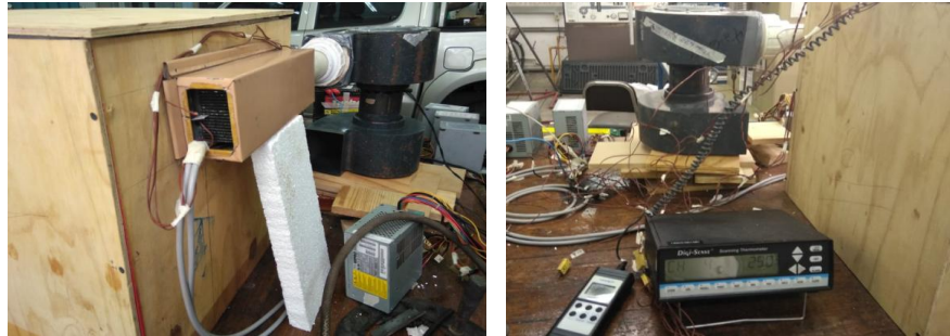
Fig. 12. Thermoelectric air conditioner placed inside of testing enclosure
