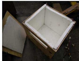
Fig. 7. Enclosure for test of thermoelectric air conditioning system
