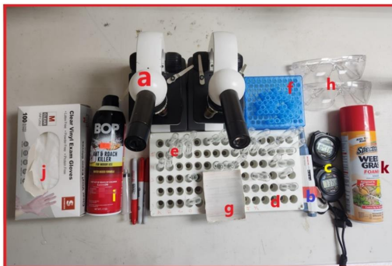
Fig. 1. The experimental materials used for the study (a: compound microscope, b: Eppendorf pipette (100~1000 ul capacity), c: stopwatches, d: tube rack, e: test tubes, f: pipette tips, g: slide glasses, h: safety goggles, i: insecticide, j: disposable gloves, k: herbicide)
