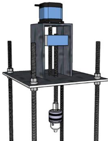
Figure (2b): the movable crosshead and mechanical linear actuator.
