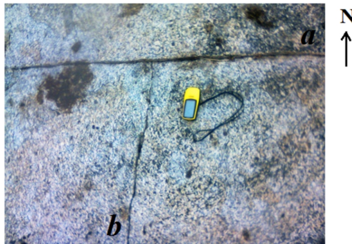
Fig. 5. Termination relationship between 'a'(E-W) and 'b'(N-S) joints in the granite. The 'b'(weaker) joint could not propagate across the void space already created by the 'a' joint which is older, stronger and wider
