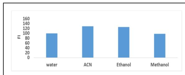
**Figure 3.** Effect of diluting solvents on the FI of 5ng/mL TEDP solution.
