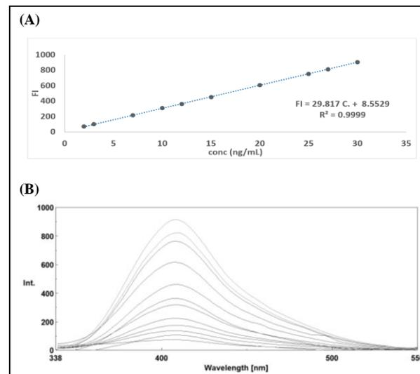
**Figure 6. (A) Calibration curve of 2-30 ng/mL aqueous solution of TEDP. (B) Emission spectra of aqueous solution of TEDP 2-30 ng/mL.**
