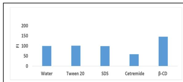
**Figure 4.** Effect of fluorescence enhancers on the FI for 5ng/mL TEDP aqueous solution.
