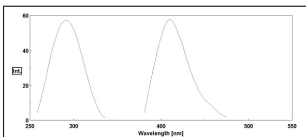
**Figure 2.** Excitation and emission spectra for 2 ng/mL TEDP in aqueous solution.
