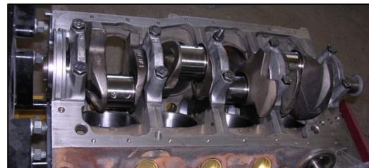
Fig. 10. Crankshaft mounted on engine
