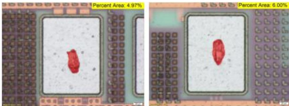
Fig. 5. Standard probe marks
