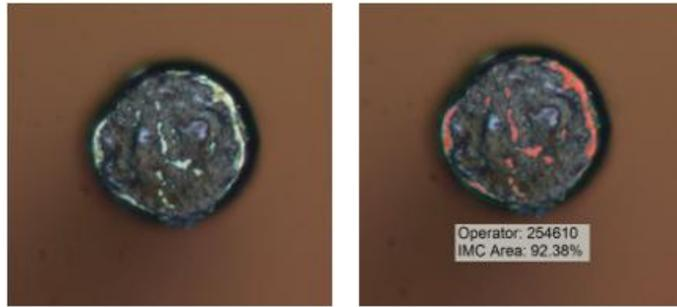
Fig. 7. IMC of standard probe mark
