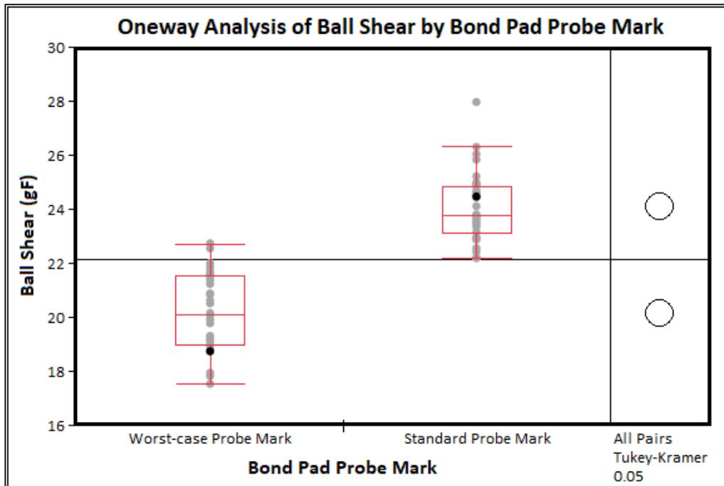
Fig. 6. Ball shear result
