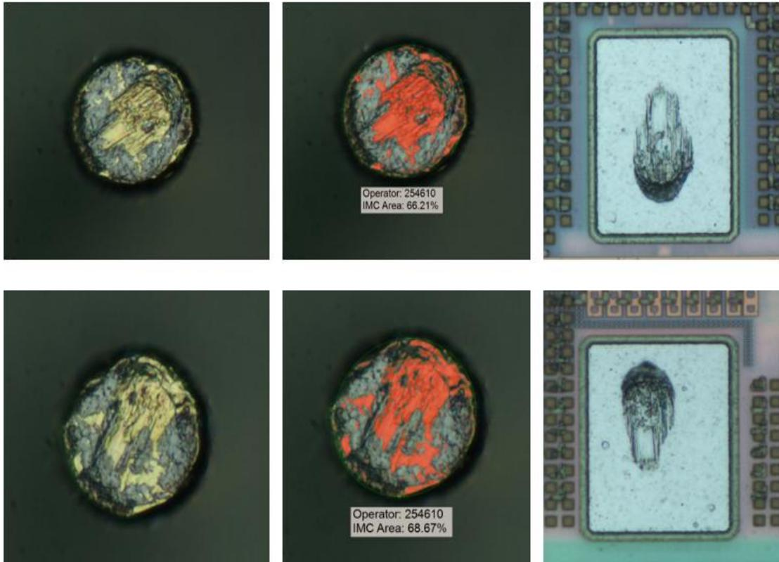
Fig. 1. IMC measurement of ball bond and snapshot of delamination on bond pad
