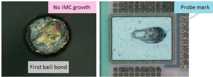
**Fig. 2. Defect signature**
