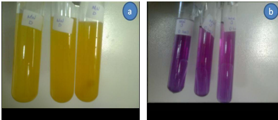
Fig. 1. Test tubes showing (a) positive and (b) negative MPN-presumptive test for coliforms, fecal coliforms and E. coli
